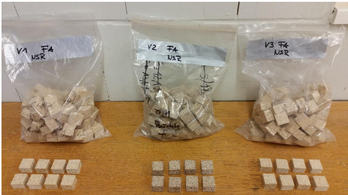
Figure 33. Samples for the determination of extractable formaldehyde and formaldehyde release of the manufactured PB models.
