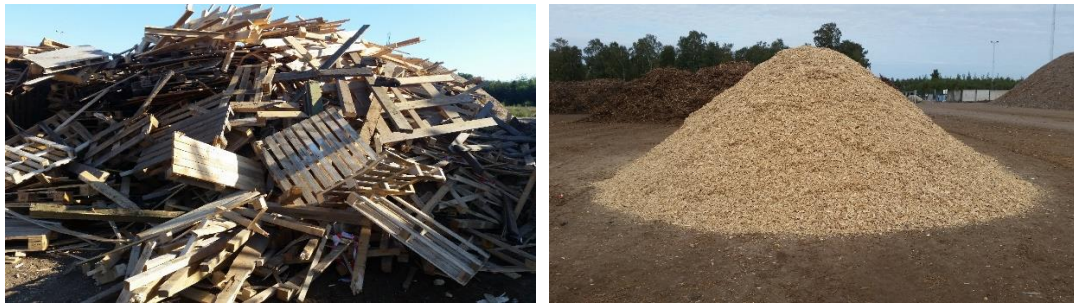
Figure 8. Unpainted wood waste, before and after crushing
