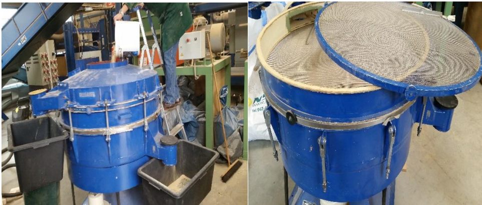
Figure 16. A Laboratory Tumbler-sift machine; ALLGAIER.
