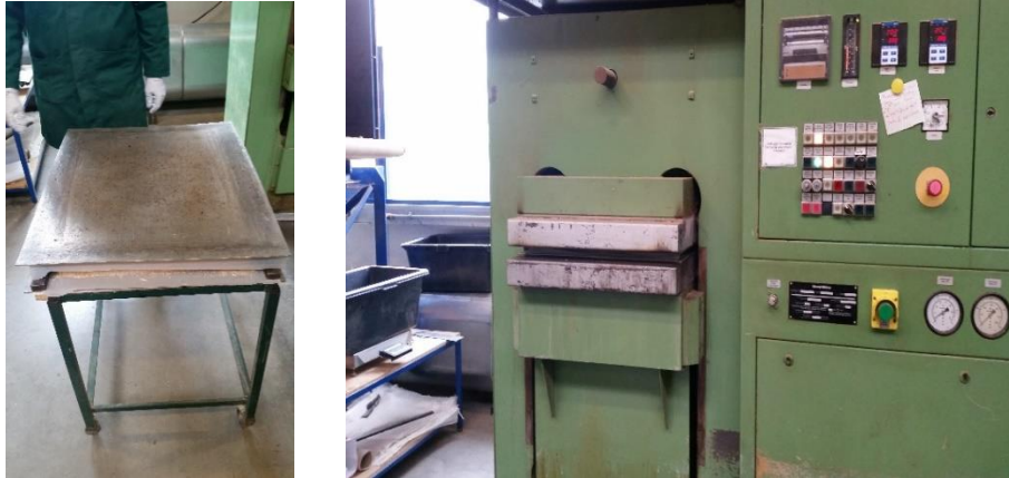
Figure 22. The mat was hot pressed using Laboratory press, Siempelkamp.
