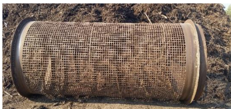
Figure 12 Meshes, 40 mm and 10 mm to Doppstadt drum sift
