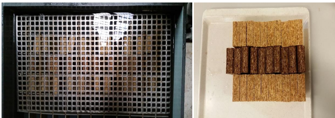
Figure 27. Soaking specimens in water at room temperature for 2 and 24 h.
