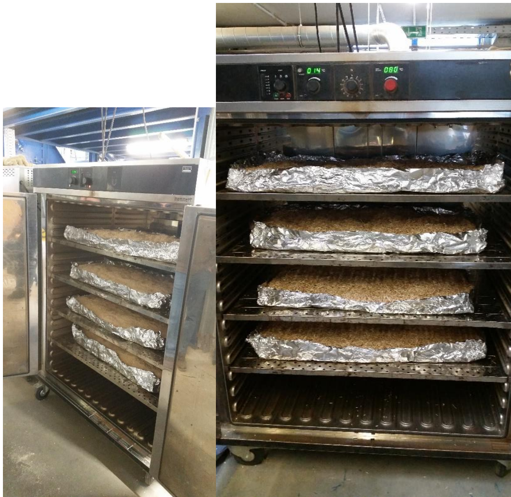
Figure 19. Drying of the wood particles at 75°C.
