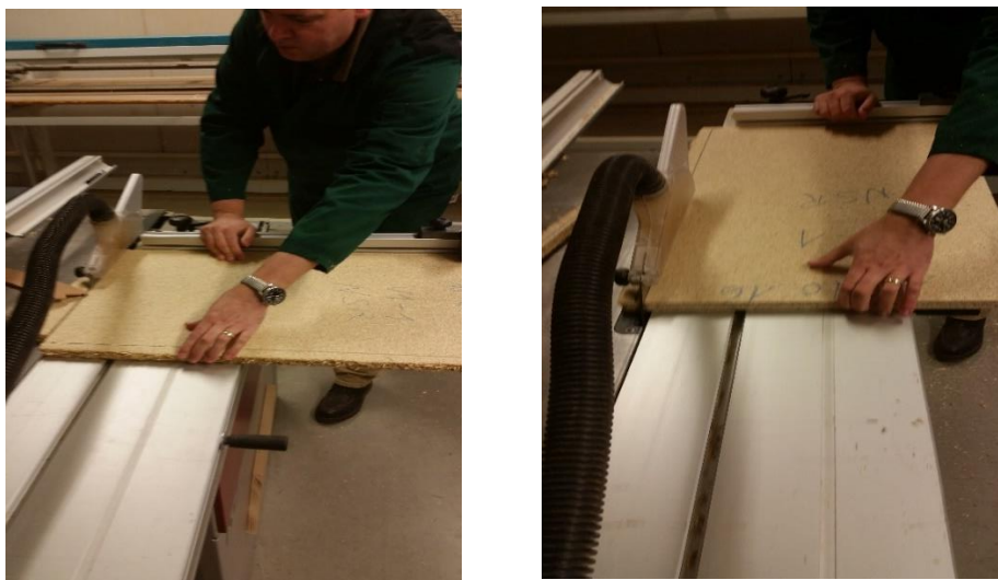
Figure 23. Trimming the manufactured models of particleboard.
