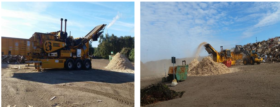
Figure 9. A CBI Magnum Force 6400 was used for crushing the wood waste (three times)
