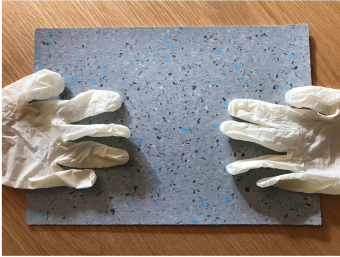
Figure 10. The produced compound (in bag) containing 20 % of pre-treated and recycled PVC from vinyl gloves and a produced floor sample partly based on the compound.
