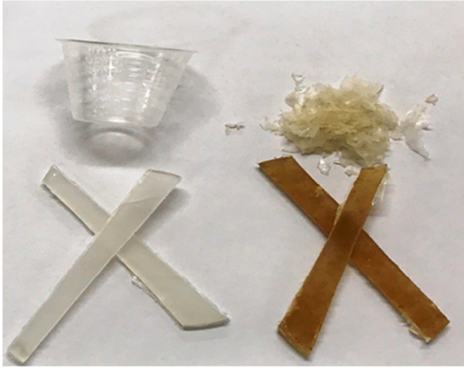
Figure 5. Comparison of visual appearance of un-treated medicine cup and remelted bars (left) with flakes and remelted bars after hydrothermal treatment (RBS)
