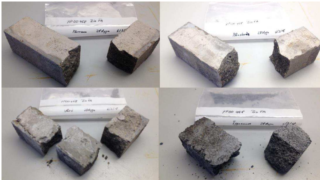
Figure 12. Bio-Fly ashes after compressive strength test at 28 days
