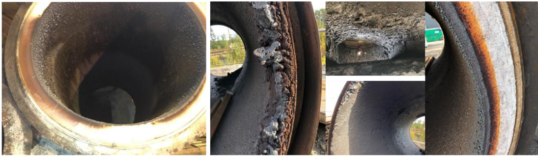
Figure 11. Figure to the left, reactor shaft after campaign 1. The other figures are of the reactor shaft after campaign 2.
