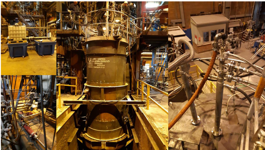
Figure 1. OXYFINES pilot trials set-up with the reactor (middle), burners through the lid at the top (right), pump (bottom left) and IBC containers (top left).
