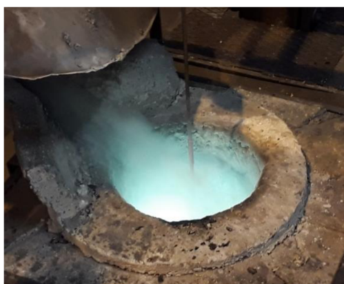
Figure 8 Induction furnace in operation during air injection tests
