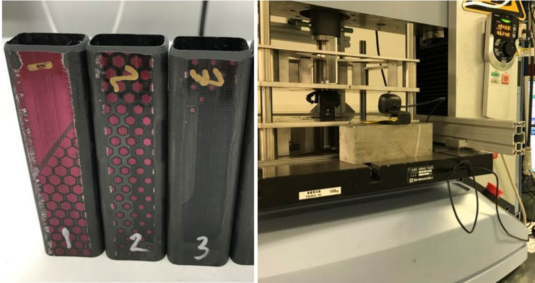
Figure 6 Examples of 100 mm long shaft sections with 30° bevel trigger introduced at one end (left) and photograph of crushing test setup (right).
