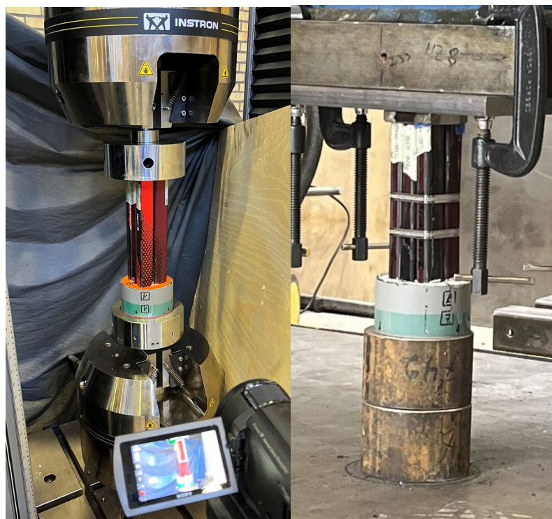
Figure 10 Photographs of test setups for crushing tests of multi-shaft sections: In the Instron 250 kN testing machine (left) and in the machine “Rörpressen” (right).
