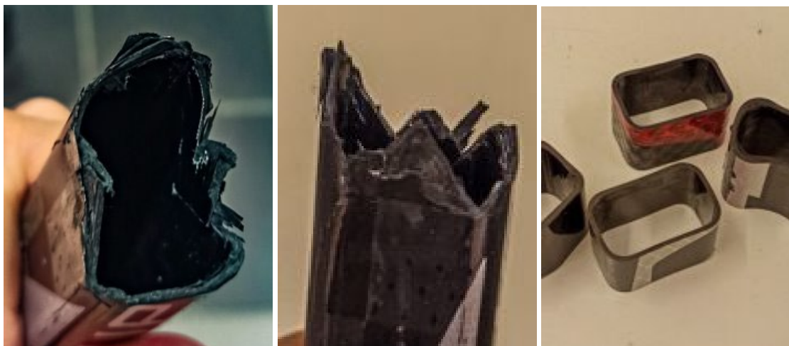
Figure 3 Photograph of broken stick section (left and middle) and cut-outs from scrapped sticks with various cross-sections (right) [1]
