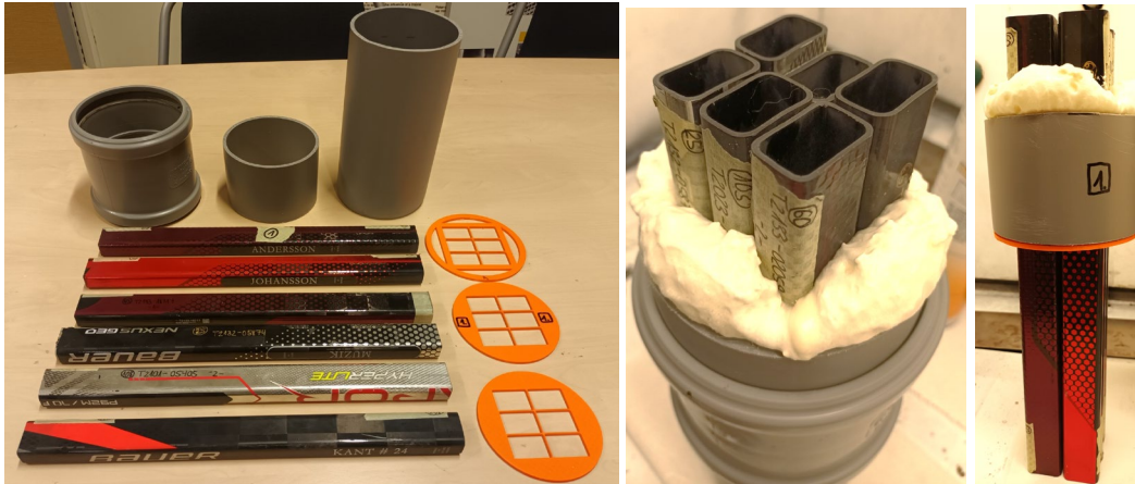
Figure 9 Items used for preparation of multi-shaft test specimens (left) and illustrating shaft sections (middle) and prepared sample before cutting base (left)
