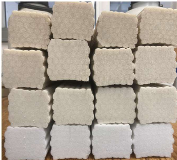
Figure 40 Foaming test performed at DIAB. Samples from top contain 75%, 50%, 25% and 0% rBHET PET.
