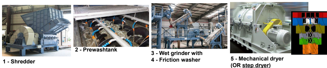
Figure 15. Washing PC-PET at Herbold Meckesheim GmbH: shredder, prewash, wet grinder with friction wash and mechanical drying.
