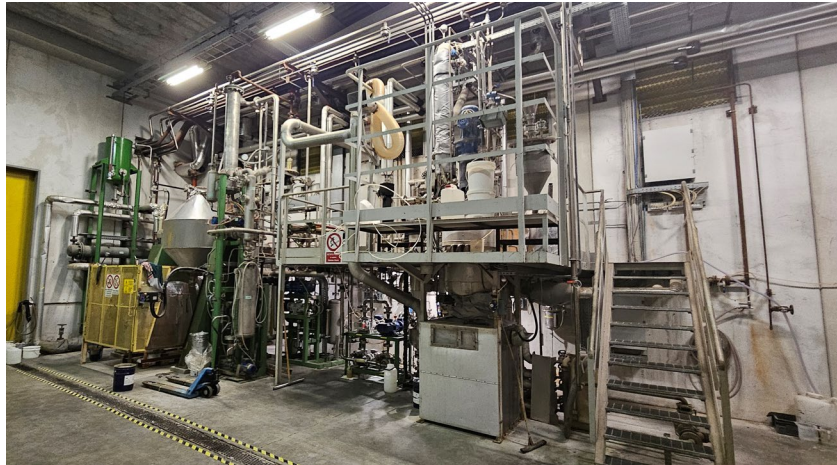
Figure 34. Pilot plant used for polymerization of BHET performed at Selenis.
