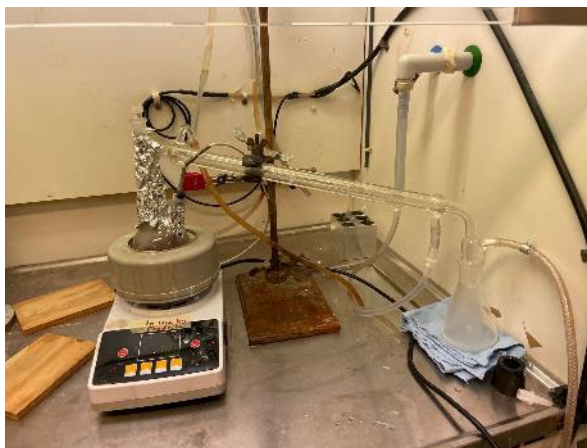
Figure 5. Experimental set-up for evaporation of ethylene glycol from reaction solution at 180°C.
