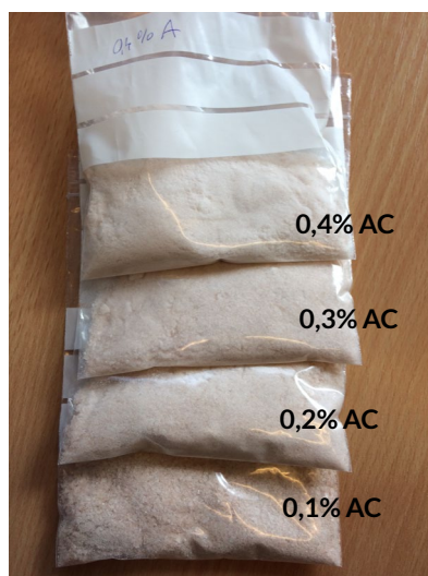
Figure 8. BHET decolorized by active carbon. The amount of carbon is given as as percentage of the weight of BHET treated.
