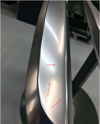
Figure 32. Surface defects Rear trim list.
