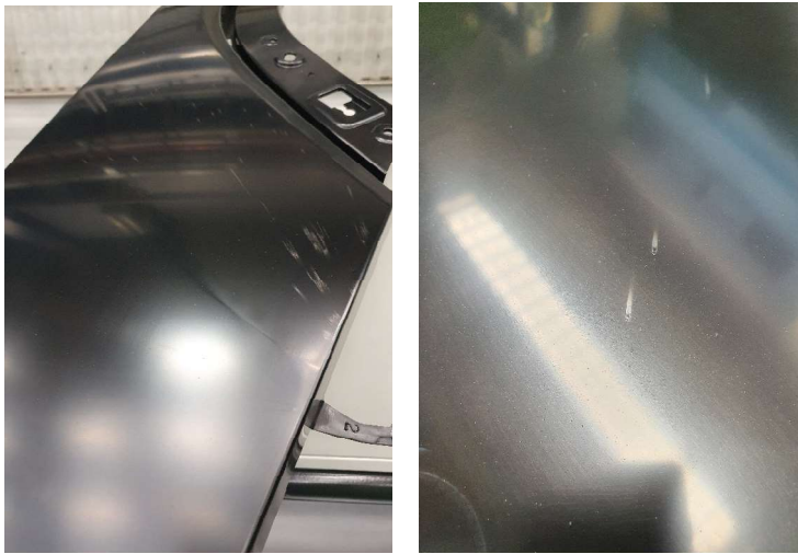
Figure 35. Some surface defects observed on the parts.
