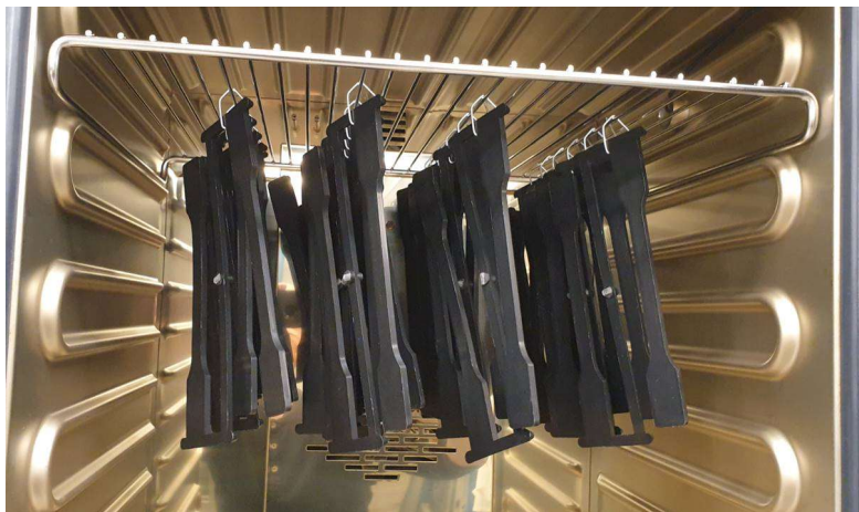
Figure 13. Test samples hanging in cabinet oven.
