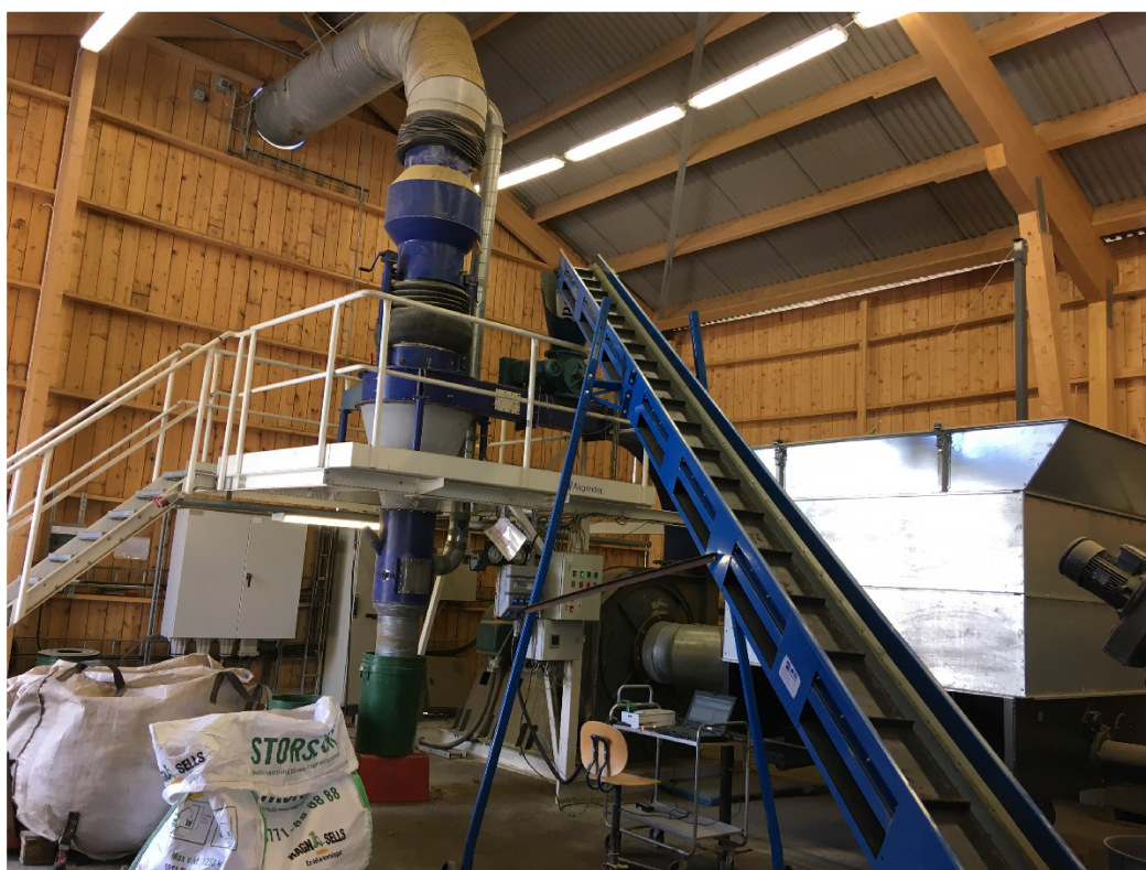
Figure 1. Cyclone dryer “Airgrinder” used for processing of fibre reject.
