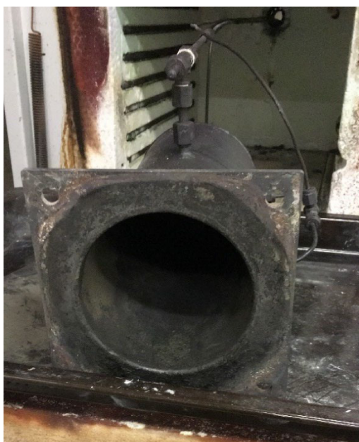
Figure 2. The reactor used for the production of activated carbon
