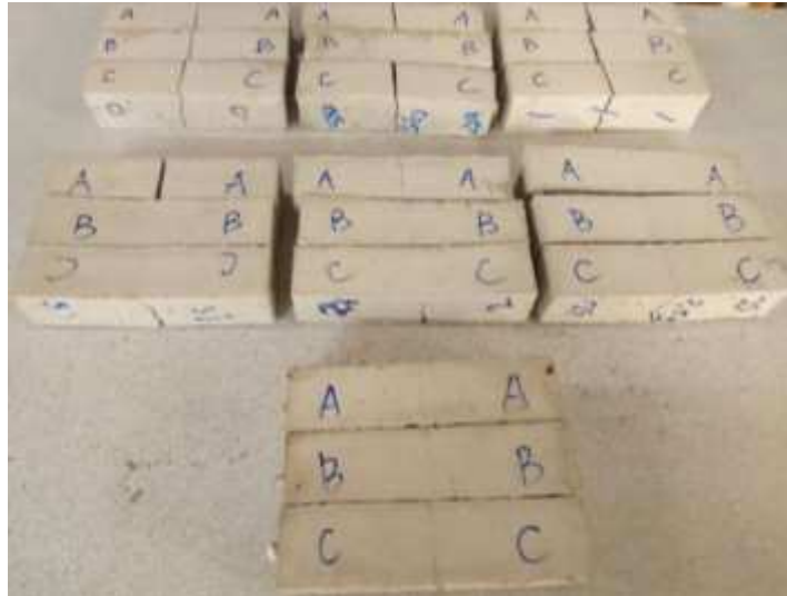
Figure 5. Cementitious mortars containing FRP granulated fillers at different fractions.
