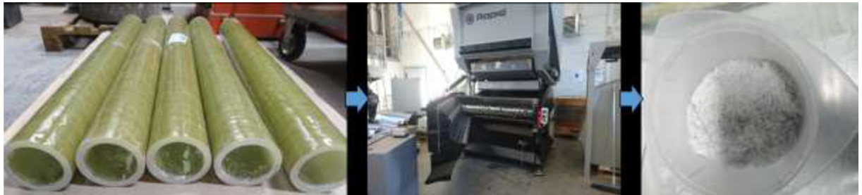
Figure 2. Granulation procedure to produce FRP fillers for cementitious and polymer matrix composites.
