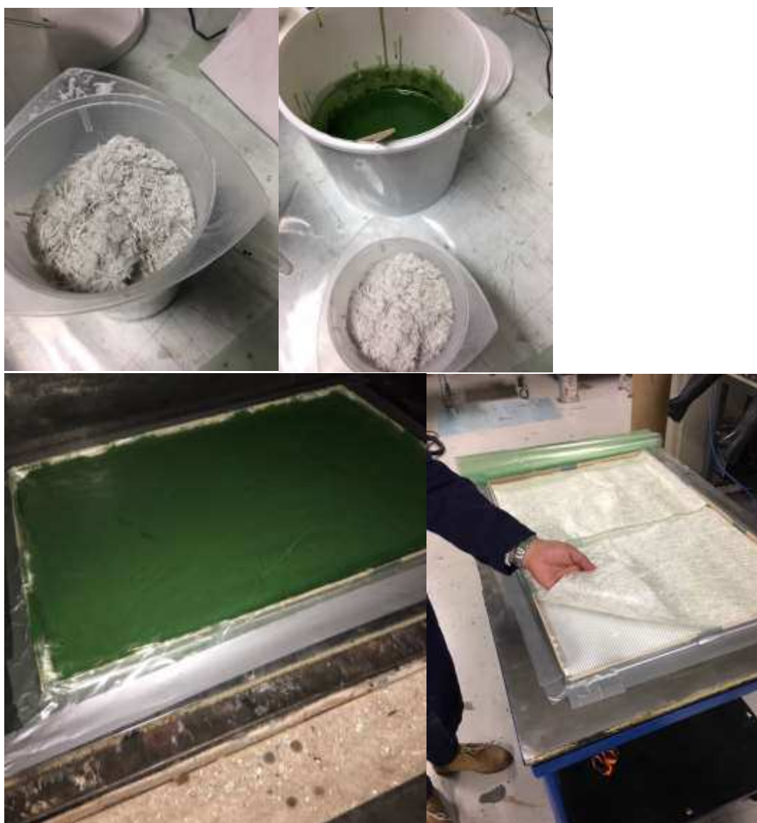
Figure 1. Resin mixture is prepared including recycled fraction. Two layers of glass fibre mats are added on top and bottom. The laminate is then cured in room temperature in atmospheric pressure. The laminate is sealed with a bag to prohibit styrene evaporation during curing.
