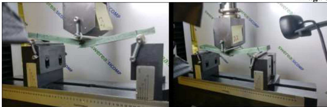
Figure 7 Specimen S3 and specimen D2 after failure
