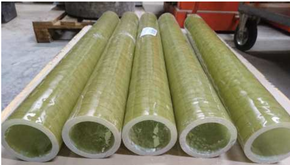
Figure 1. Discarded FRP insulation pipes from ABB Composites AB that were ground and used as filler in cementitious and polymer matrix composites.
