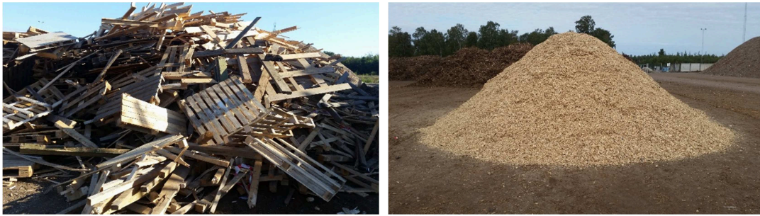
Figure 8. Unpainted wood waste, before and after crushing
