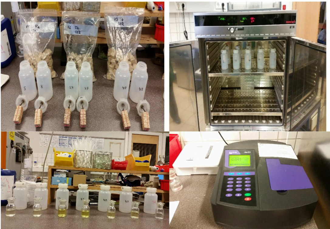
Figure 35. Determination of formaldehyde release acc. To WKI-flask- method, EN717-3 from the manufactured PB models.
