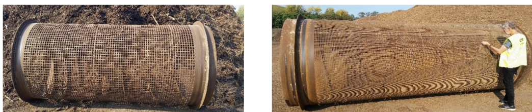
Figure 12 Meshes, 40 mm and 10 mm to Doppstadt drum sift
