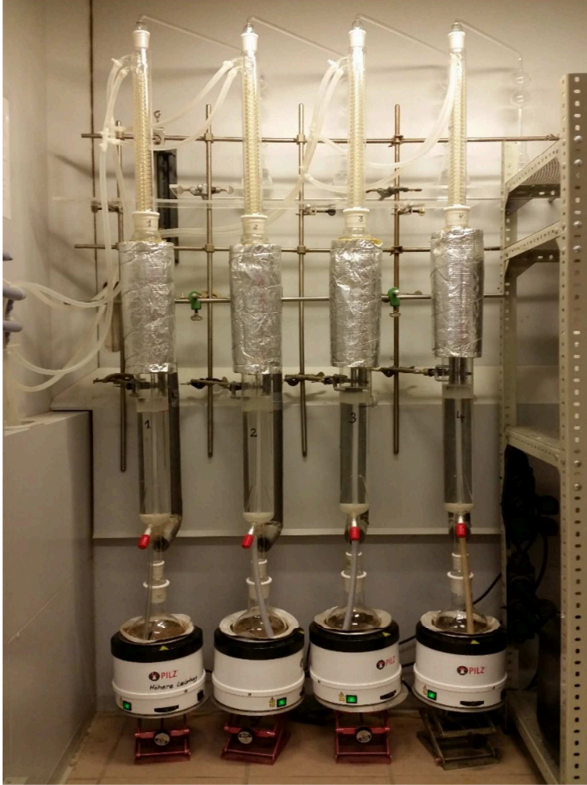
Figure 34. Determination of extractable formaldehyde acc. to perforator method, EN 120 from the manufactured PB models.
