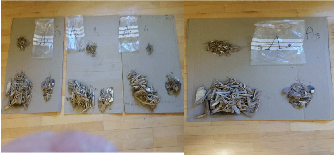
Figure 6. The sample's components: Wood chips of massive wood, wood chips of manufactured wood (particleboards or other wood based panels), and fines and other impurities
