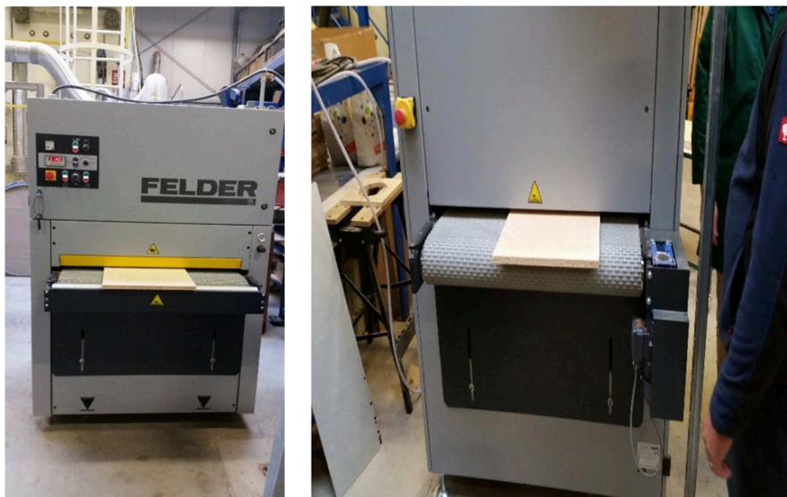
Figure 24. Sanding the manufactured models of particleboard.
