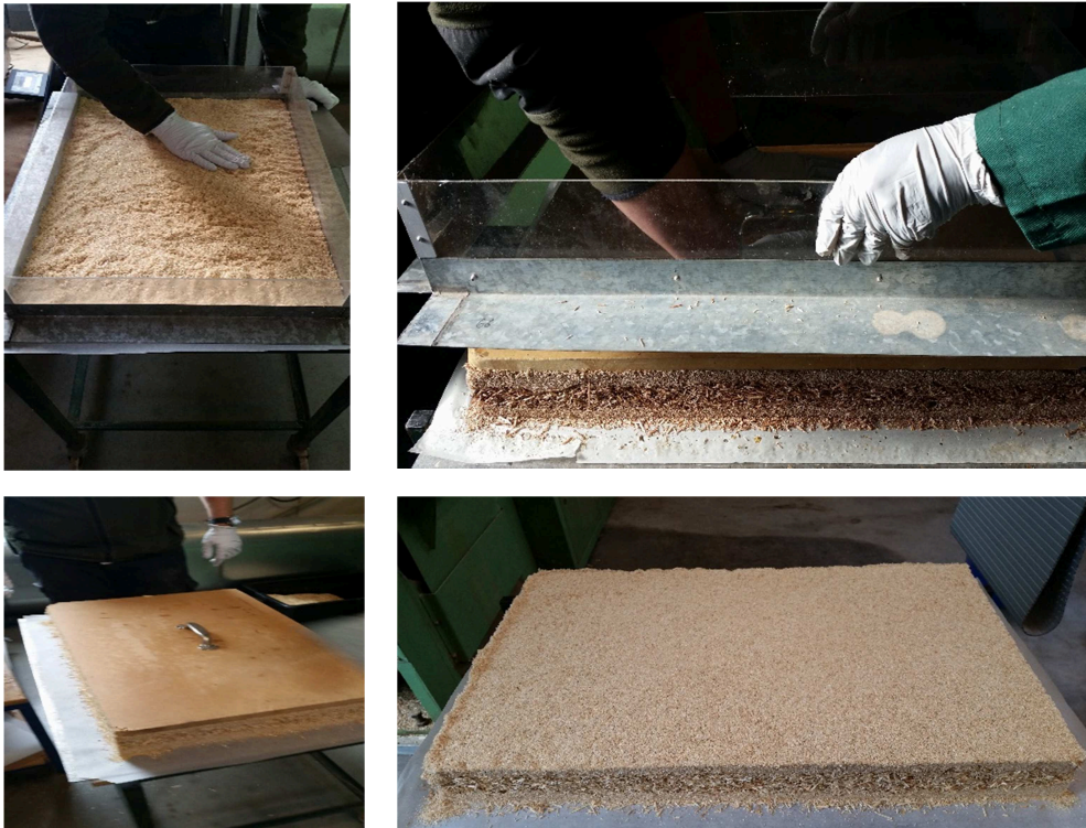
Figure 21. Forming the board, the mixed particles were hand-felted into a frame 70 x 45 cm on metal plate and pre-pressed by hands.
