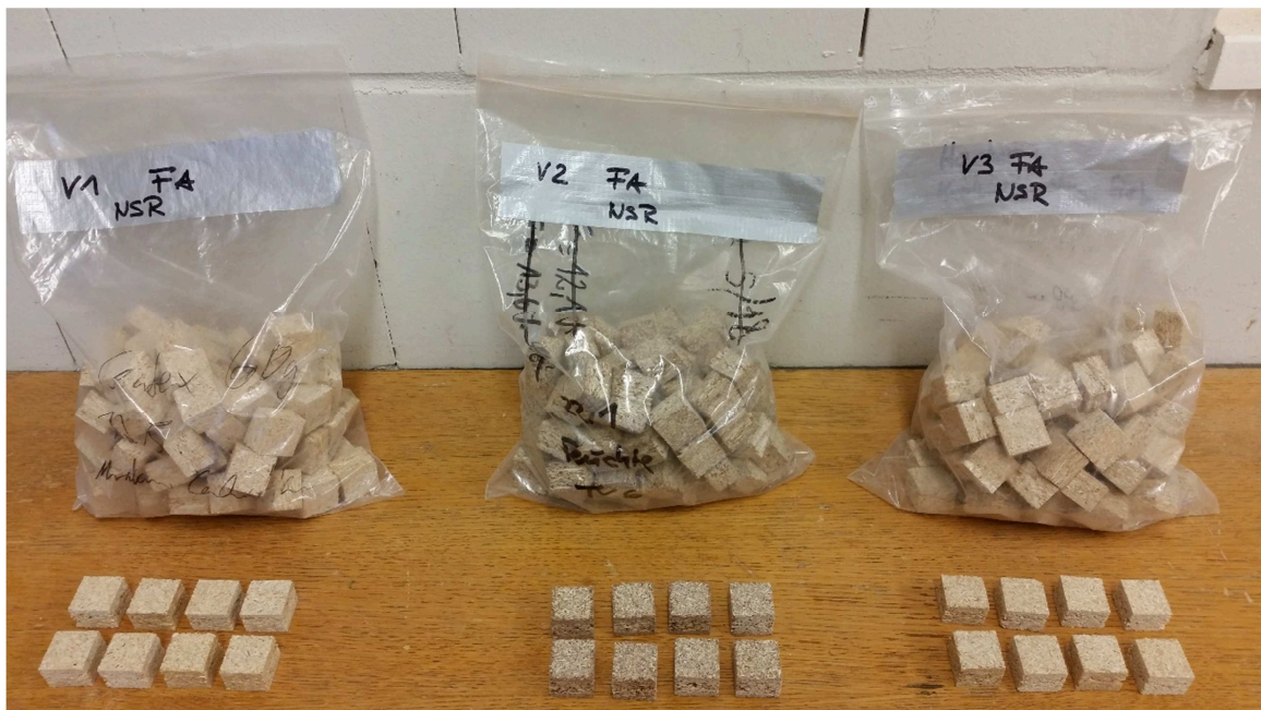
Figure 33. Samples for the determination of extractable formaldehyde and formaldehyde release of the manufactured PB models.
