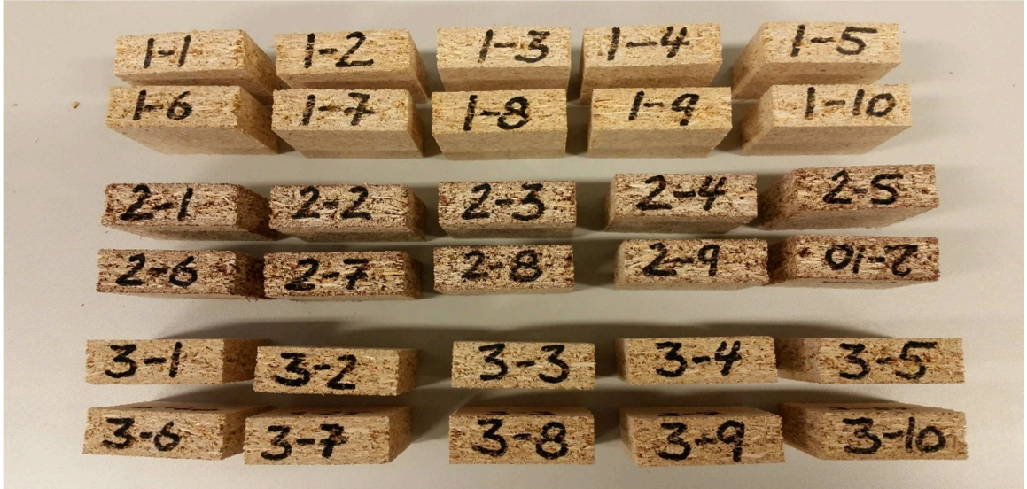
Figure 30. Samples for determination of internal bond (IB) strength (EN 319).
