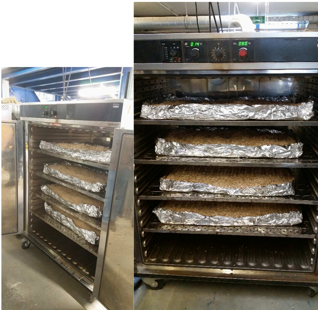
Figure 19. Drying of the wood particles at 75°C.
