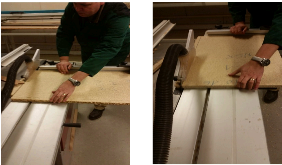
Figure 23. Trimming the manufactured models of particleboard.
