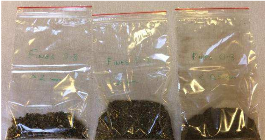
Figure 15. The final samples of NF-fines fraction used to produce the epoxy mounts. Left: > 2 mm, center: 0.5 - 2 mm, right: < 0.5 mm.
