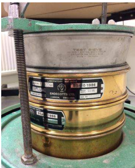
Figure 12. The sieving equipment. The sieving time differed from fraction to fraction and was stopped after visual inspection not after certain time span.
