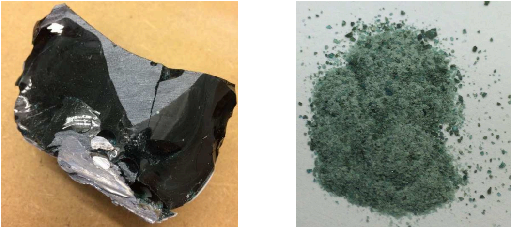
Figure 7. To the left: crucible divided with diamond saw, the glass phase and the lead phase can be seen. To the right: glass phase crushed with a mortar and pestle.
